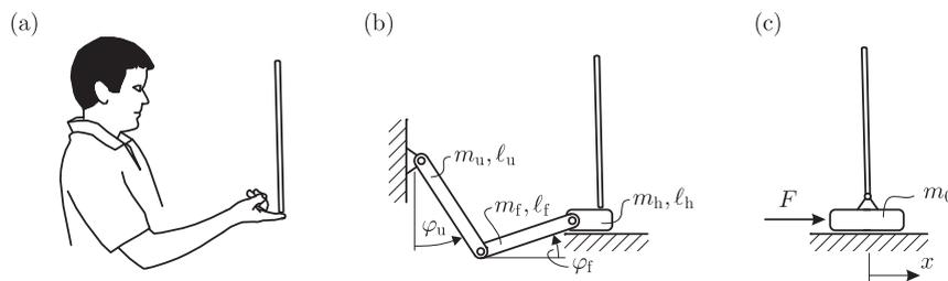
Fig. 1. Model of human arm mechanism.
