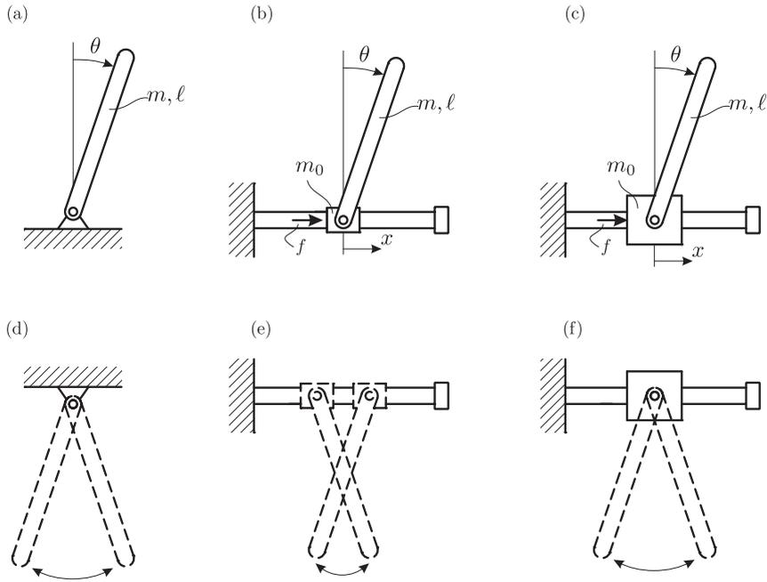
Fig. 2. Mechanical model of (a) pinned pendulum; (b) pendulum-cart model with negligible cart mass ( $m_0 \ll m$ ); (c) pendulum-cart model with  $m_0 \gg m$ . Panels (d), (e), (f) shows the oscillations when the pendulums are hung downward.
