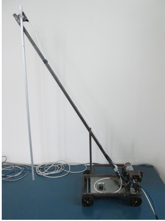
FIGURE 4.3. Mobile crane experimental device
